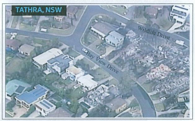
Note the destruction in Bay View Drive. These houses are zoned as NOT being **Bushfire Prone**. Note also the absence of damage to houses in Wildlife Drive notwithstanding that they abut the bushland at the top of the image and are zoned as **Bushfire Prone**, a dramatic illustration of the difficulty of predicting liability to bushfire damage.
